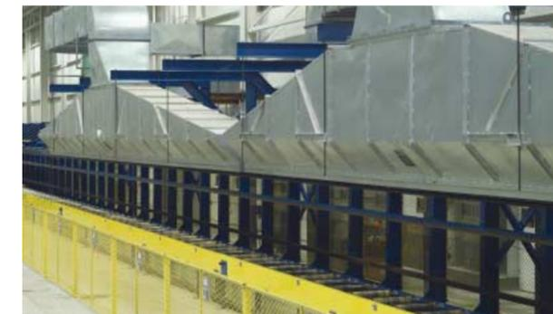
Granco Clark’s Overhead Cooling Duct System creates a continuous “curtain” of cooling air over the runout conveyor.
