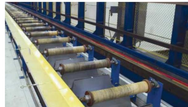
Granco Clark’s Integral Runout Cooling System features distribution ducts within the runout table.
