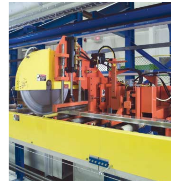
On the Granco Clark Twin Puller, an adjustable hot saw cuts the profile during the dead cycle.
