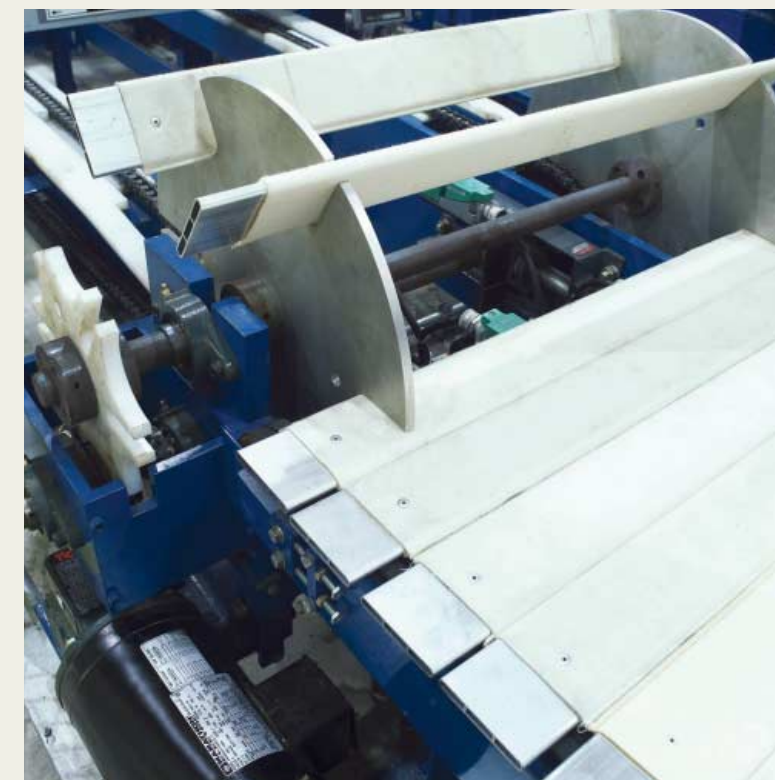
Spacers are automatically inserted, saving time and labor.
