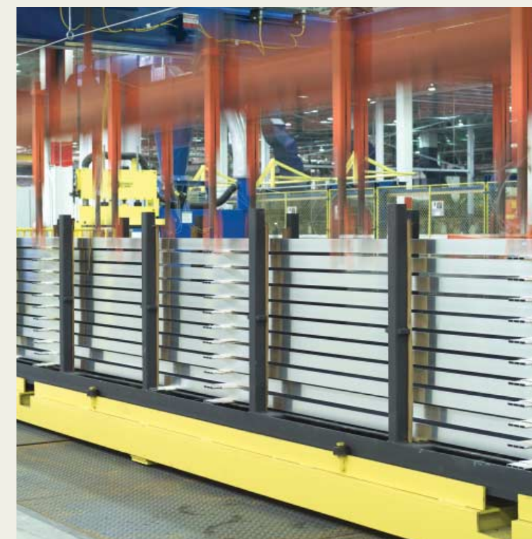
Granco Clark automatic stackers rapidly offload extrusions from the gauge table to aging racks.
