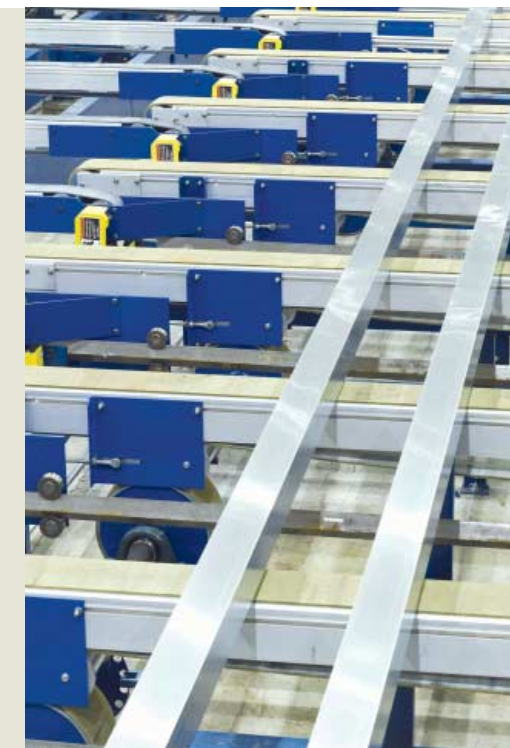
The cooling belt table provides a mark-free surface for profiles to rest on as they cool, preserving profile surface quality.
