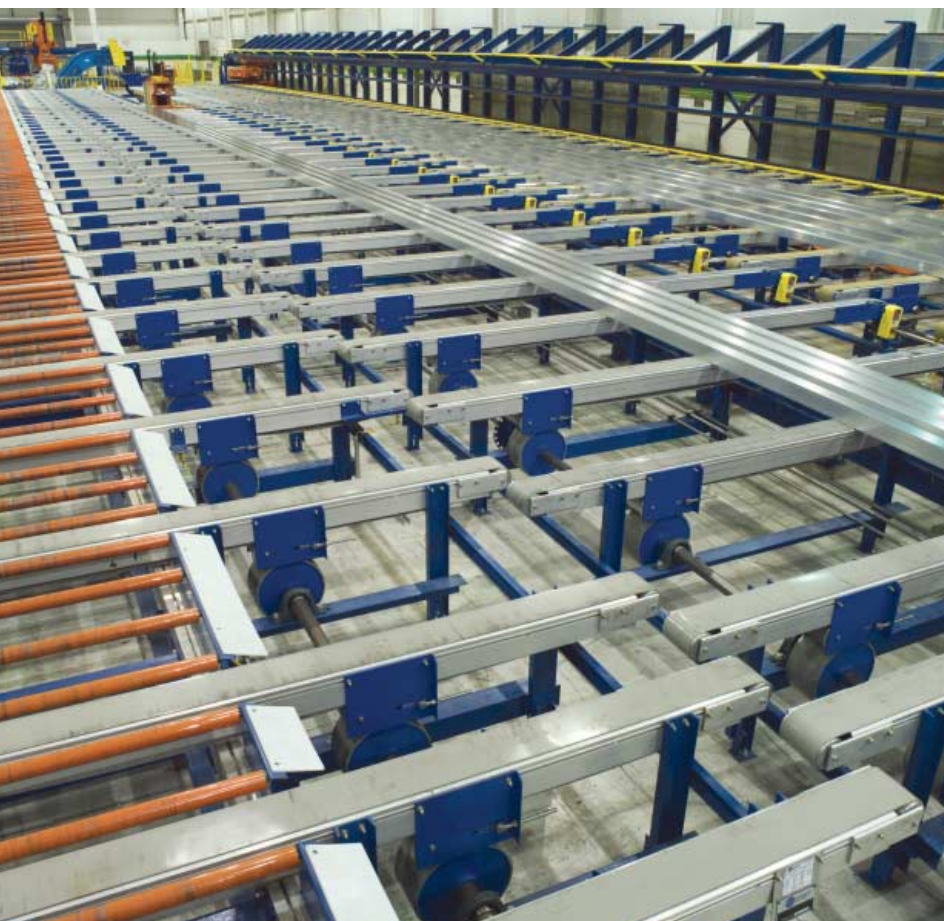
Granco Clark's batching, storage, and saw-feed loading-belt system automatically receives extrusions from the stretcher, batches them, and feeds them into the saw.
