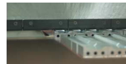
Horizontal and vertical clamps completely enclose product. THK slide guides provide firm, even pressure and eliminate guillotining.
