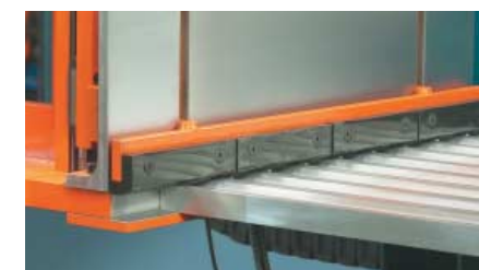
Backgauge clamping exerts positive control over extrusions, providing the fastest cycle times in the industry.
