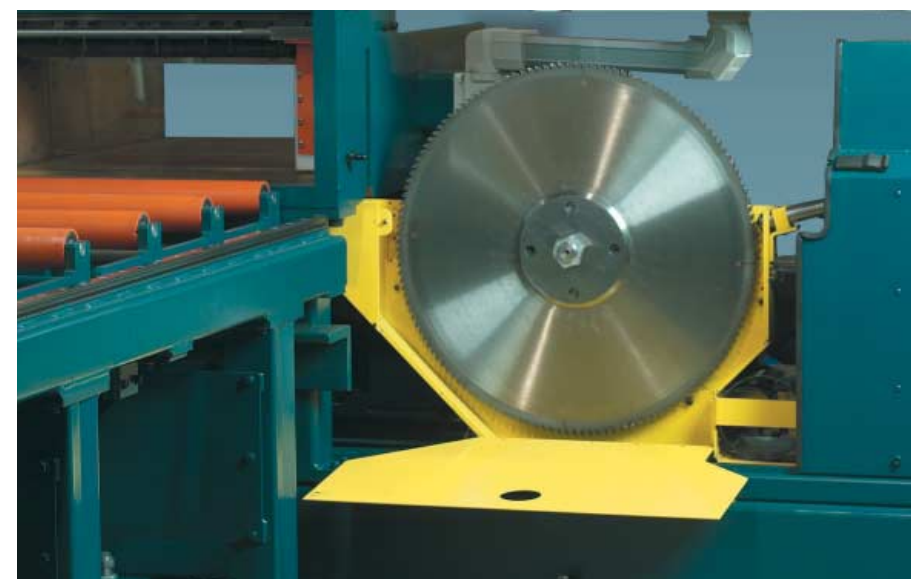
The Granco Clark Precision Finish Saw features the industry's only blade carriage screw design, providing increased precision. The saw's design makes maintenance a breeze. All moving parts are easily accessible. The blade housing easily rolls back, minimizing blade change time and simplifying access for continuing care and adjustments.
