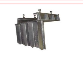
The ScrapEater can be mounted on your floor or furnace sill. The above mounting plate is used when attaching the ScrapEater to the furnace sill. The mounting plate is welded onto the furnace sill. The ScrapEater can then be placed into the bracket using a forklift and bolted down. Removal is just as easy - simply unbolt and remove the ScrapEater with a forklift.
