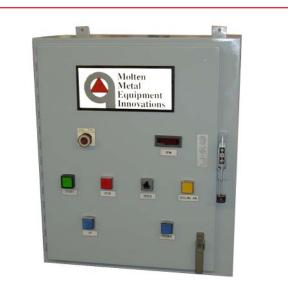
The ScrapEater controls are simple to operate. Rotational speed of the shaft and melter bottom are controlled by dial with an RPM readout. There are separate buttons for controlling up and down motion for precise placement of the melter bottom in the metal bath. Start, Stop and Emergency Stop buttons are also provided.
