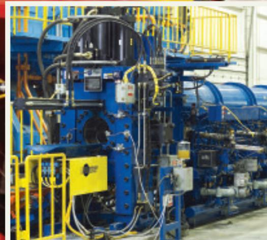
Integrated with our Hot Jet furnace, a Granco Clark Log Shear cuts billets to the desired length immediately before entering the press for maximum efficiency.
