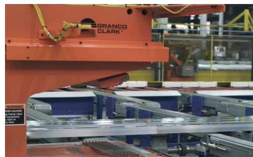
*The stretcher jaws open to accept new profile batches...*
