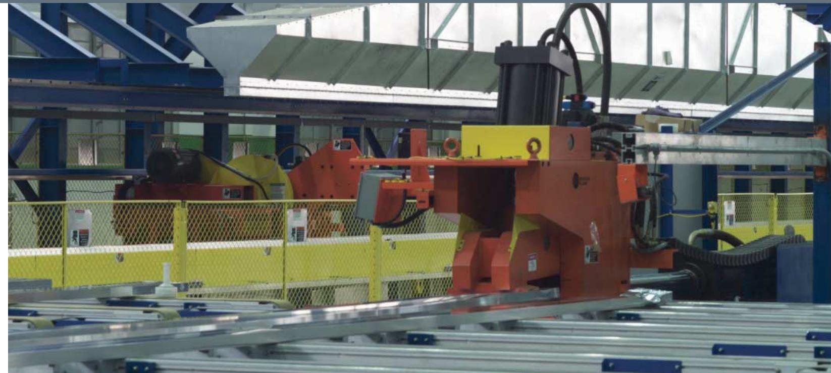
*The Granco Clark Controlled Vertical Crush Stretcher delivers maximum gripping control with minimum distortion.*
