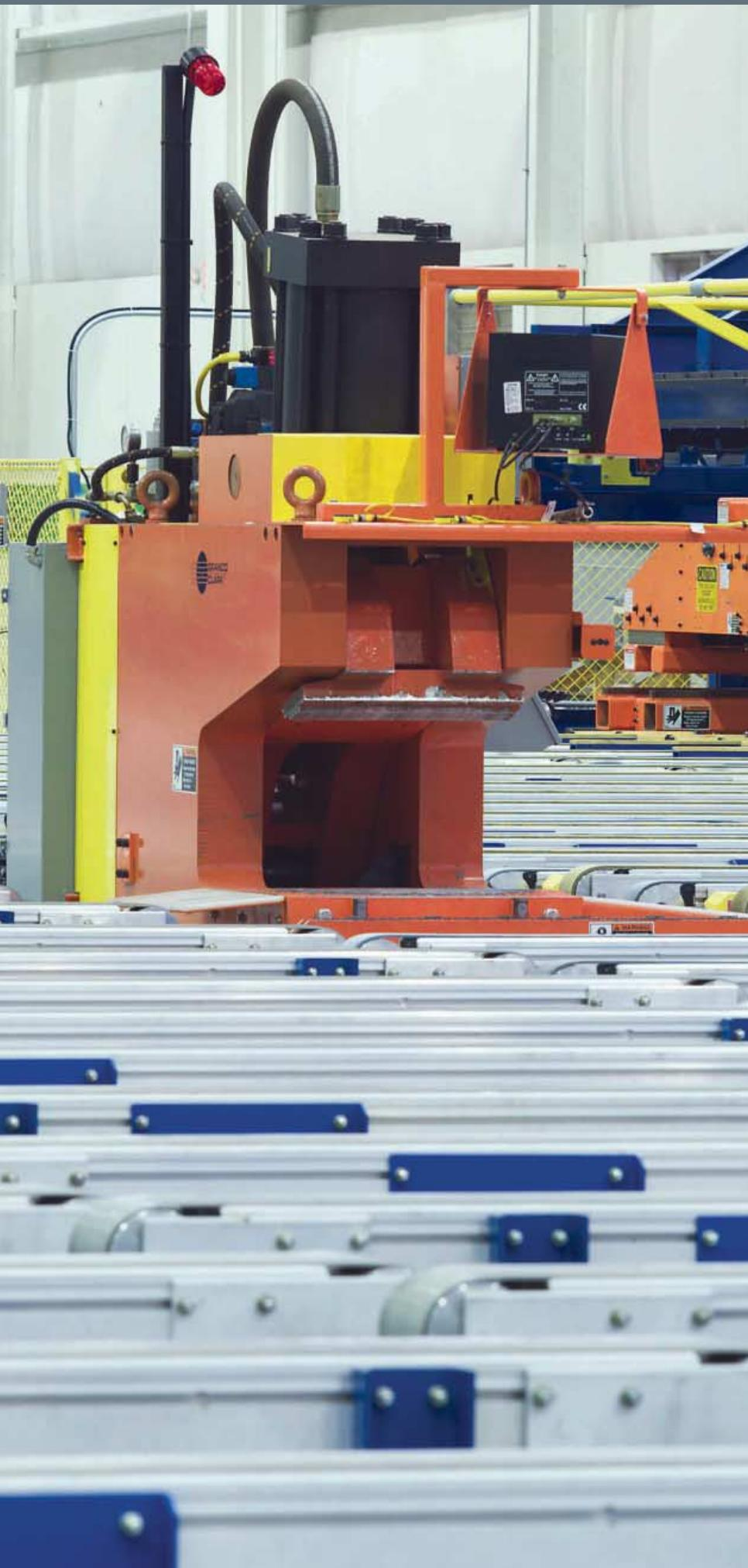
Stretching is one of the most critical post-quenching operations in the extrusion process: Performing that function correctly often makes the difference between usable product and scrap. An overstretched profile will be out of tolerance; a profile that is not stretched to its yield point will snap back unstraightened. Both are destined to become scrap.
