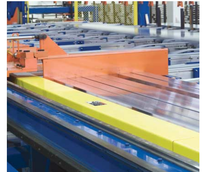
The extrusion batch moves forward until profile ends are firmly butted against the saw gauge stop.
