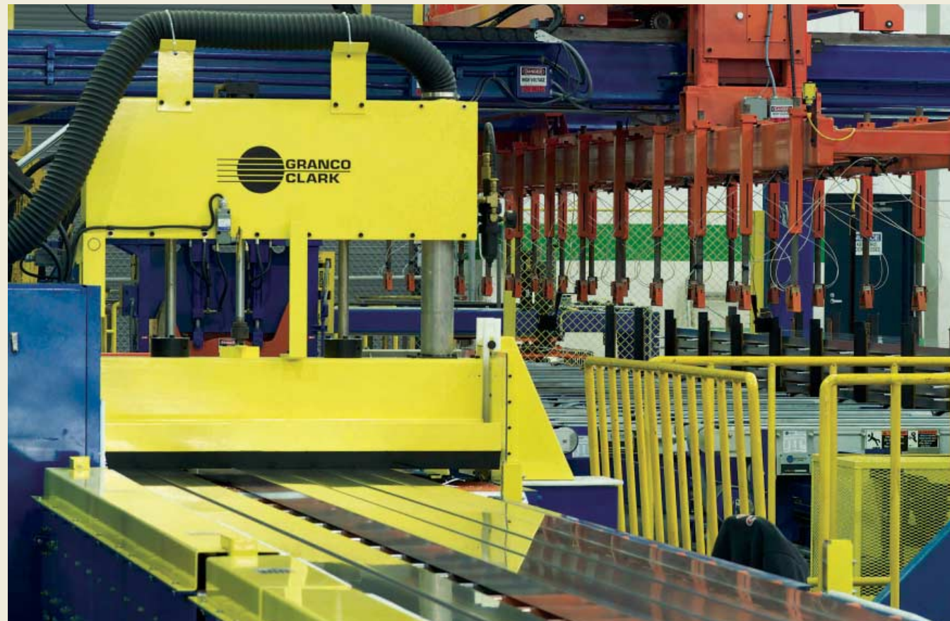
The saw hood lowers automatically to clamp the profiles.
