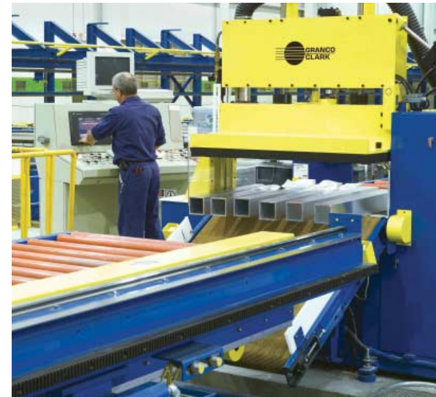
Scrap ends are automatically removed via a tilt belt conveyor.
