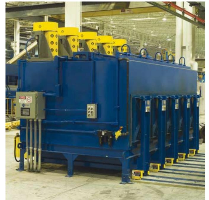
The Granco Clark multi-compartment die oven features individually heated drawers, minimizing heat loss and providing convenient die handling.
