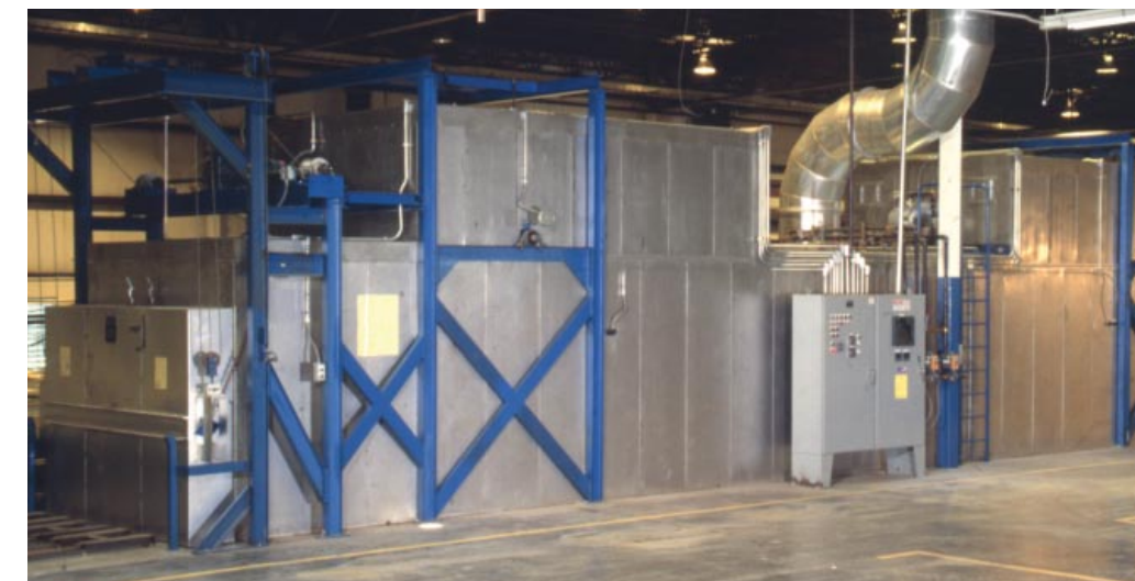
Top: The Granco Clark single-end-flow age oven provides excellent temperature uniformity for chamber lengths of up to 50 feet.
