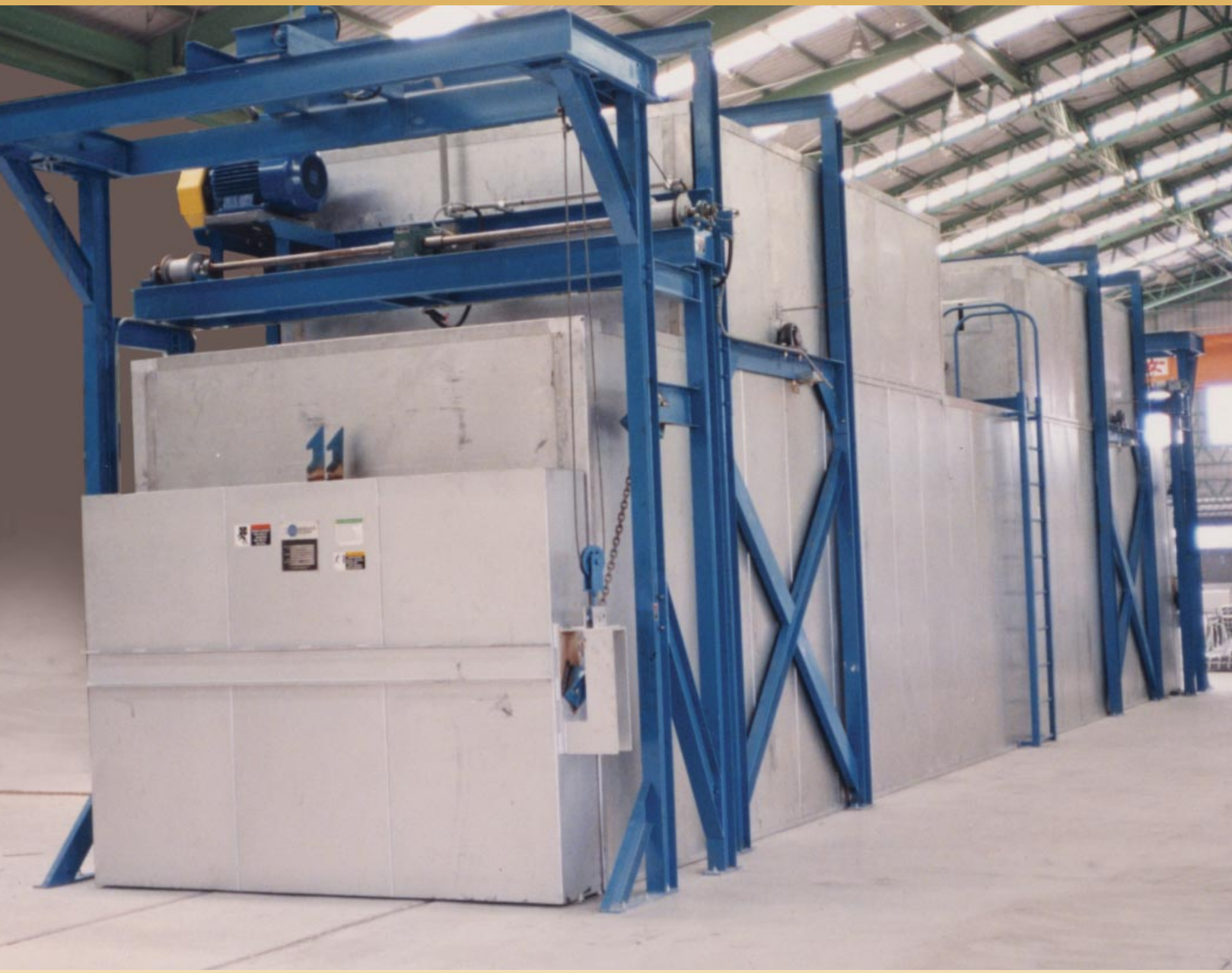
High-volume air systems bring oven loads up to temperature quickly (nominal one to two hours).
