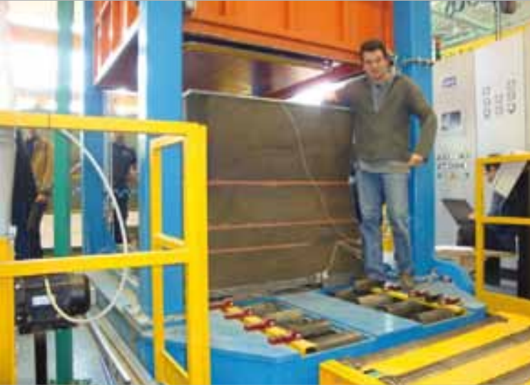
④ aluminium and magnesium low pressure sand casting machine
