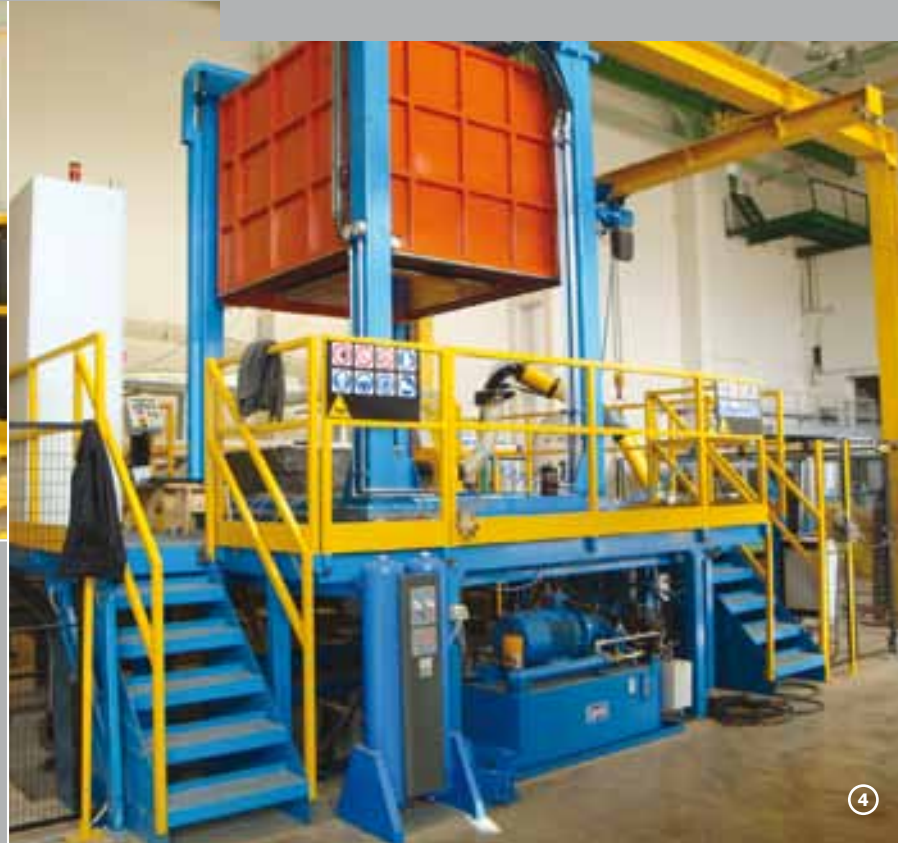
④ aluminium and magnesium low pressure sand casting machine
