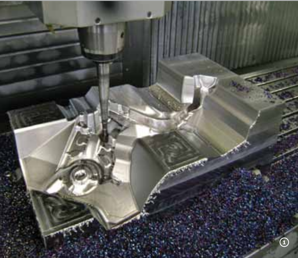
① Machining of "control arm" mold
