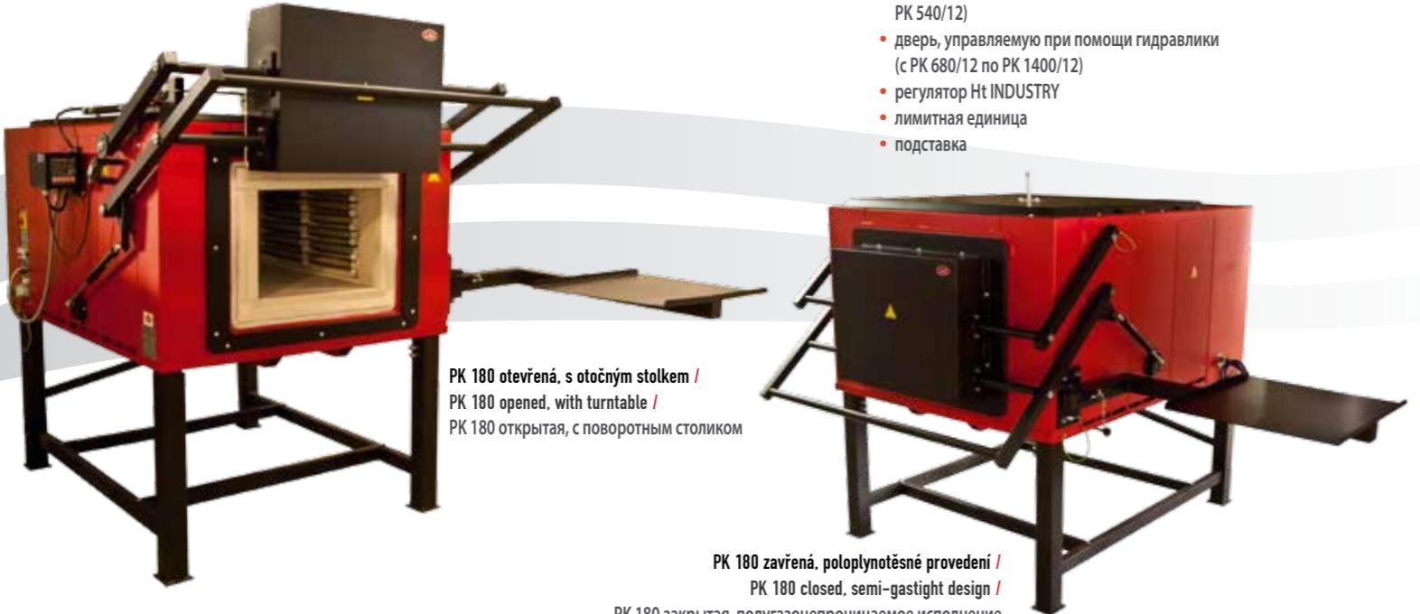
PK hardening furnaces are used especially for the hardening, annealing and preheating of metal charges before forging, in oxidizing atmosphere. Semi-gastight version PK furnaces with retort can be used for the heat treatment of the charge in partially shielding gas.
