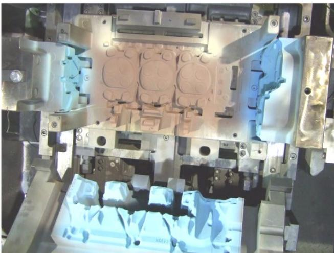
**Nanocomp V7HI** may be applied above 140°C. This avoids moisture defects on actively cooled mould sections after touch-ups.
