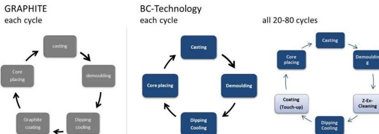
It is only after a great number of castings, that any interventions are necessary with the BC technology. The time needed for these interventions is similar to the one needed for graphite application – which is required for every single run.
